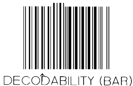
Figure 5.5.3.3.12 – 3. Calibration Symbol with Engineered Low Decodability Grade
