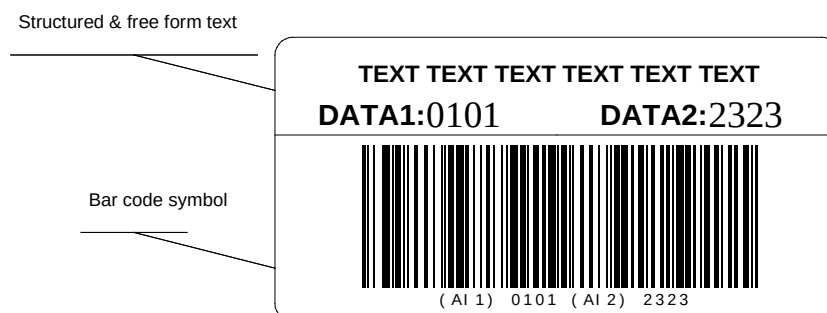
Figure 6.7.3.2 – 1. Bar code and Human Readable Interpretation Layout
